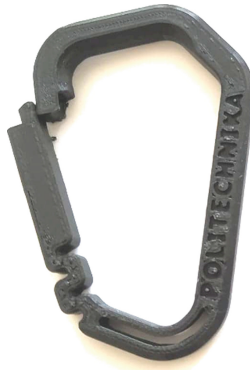
Fig. 3. Shape of the printed test product, finished product (8 cm × 5,3 cm × 0,8 cm).
