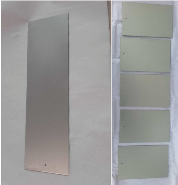
Fig. 2. Anodic oxidation using sulfuric acid after the corrosion test. From left a) material 2024 b) material 7075
