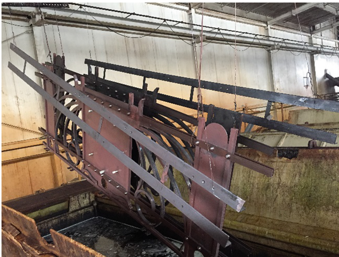
Fig. 8. Pickling before application of hot-dip zinc by immersion
