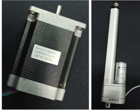
Fig. 8. Stepper motor and linear actuator used for actuating the structure
