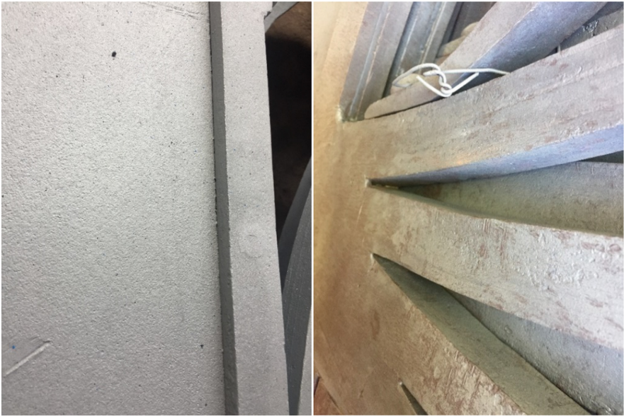
Fig. 7. Pre-treatment of the surface by blasting before application of hot-dip zinc by immersion - surface cleanliness of Sa 3 grade
