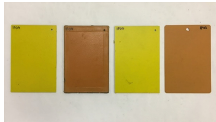
Fig. 6. Results of the second series before testing. From the left IP04 and IP03. On the left, the sample is always heated to the color transition temperature [25].
