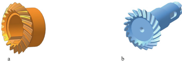
Fig. 3. Solid models of bevel gear elements: a – gear wheel; b – pinion
