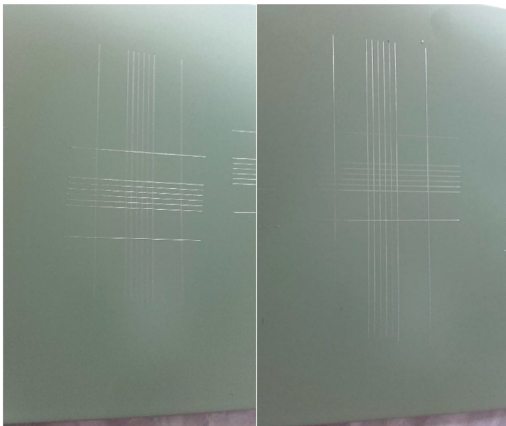
Fig. 5. Grid test: From left a) material 2024 b) material 7075
