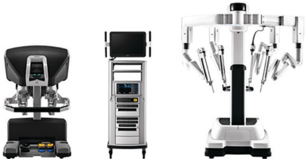
Fig. 1 The three components of the DaVinci Xi system and the surgeons console, visual tower, and patient cart on a single extendable and maneuverable boom
