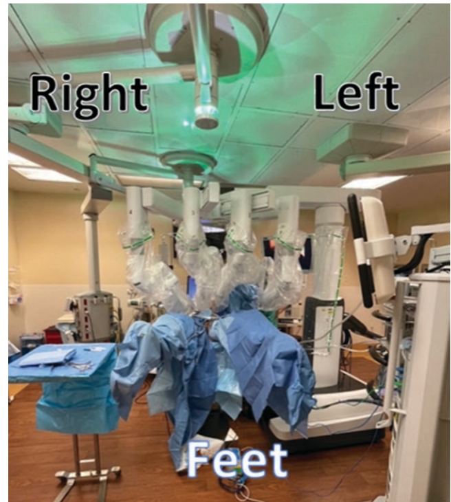
Fig. 7 View of “Side docking” from the patient’s feet. Surgical cart is at the patient’s left. (Photo courtesy R. J. Leveillee, MD, FRCS-G)
