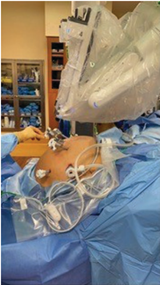
Fig. 4 Traditional docking “between the legs” with the DaVinci Xi. (Photo courtesy R. J. Leveillee, MD, FRCS-G)
