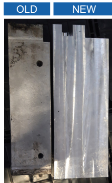
Fig. 9. Comparison of the old and new centering clamps (own study).
