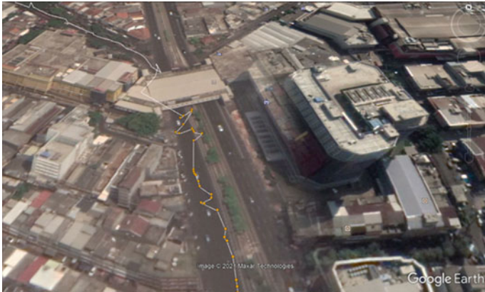
Fig. 5 Signal error in between high-rise building canyon within the underpass tunnel
