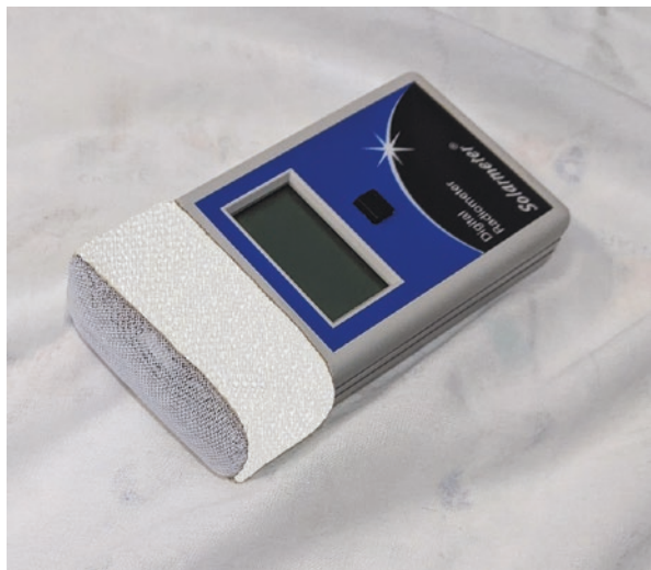
Fig. 5 Example of an irradiance meter with a mesh attached (Courtesy of Dr. Sleeth)
