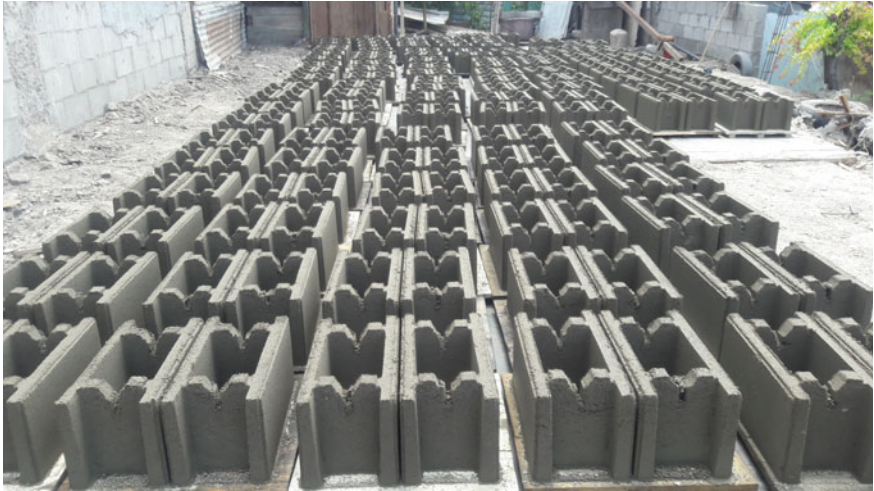
Fig. 19.5 Interlocking concrete blocks drying in the property of a participating family. Photo Monica Peralta
