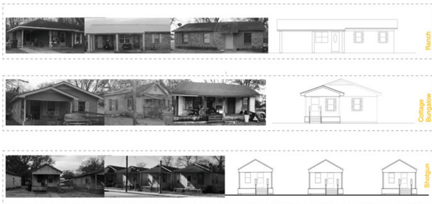
Fig. 25.3 Housing Typologies: ranch, cottage, bungalow, and shotgun. Photographs and drawings Silvina Lopez Barrera
