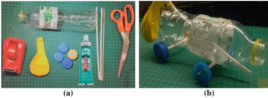
Fig. 18.2 (a) Materials for the activity “Propulsion car”, plastic bottle, straws, wooden sticks, black marker pen, silicone glue, scissors and a balloon. (b) The propulsion car already made
