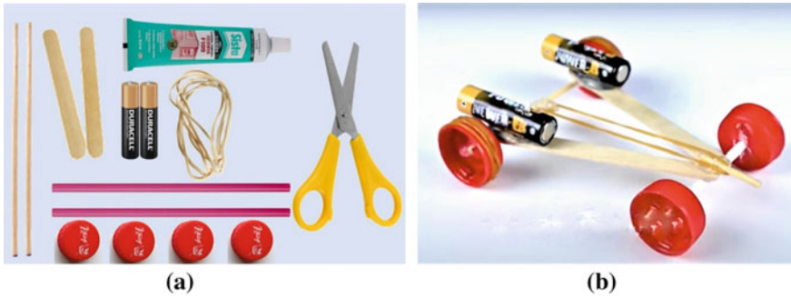
Fig. 18.3 (a) Materials to make a traction car: 2 tongue depressors, 4 screw caps, 2 plastic straws, 2 wooden sticks, silicone glue, scissors, and rubber bands, 2 discharged AA batteries. (b) The traction car already built
