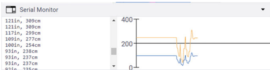
Fig. 3 Ultrasonic sensor data displayed on serial monitor of arduino IDE
