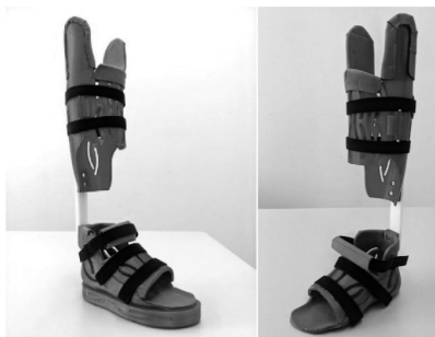
Fig. 6. The manufactured orthosis, design 1 – PET-G
