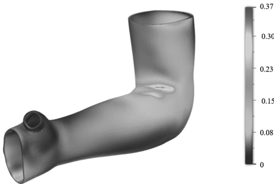
Fig. 5. Obtained von Mises stress distribution during preliminary study- stresses are expressed in [MPa].
