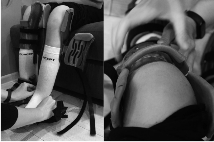
Fig. 9. Fitting of orthosis, version 1 – visible problems
