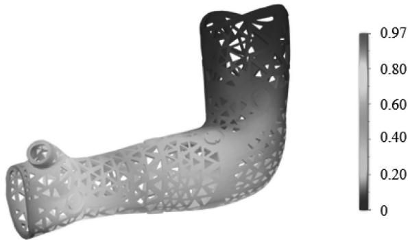
Fig. 10. The results obtained for the Case I - displacements expressed in [mm].
