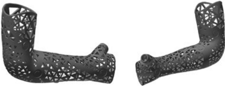
Fig. 6. Applied 3D pattern structure (triangle elements) – variable pattern elements size and distances between them depending on the level of stress in the defined area.
