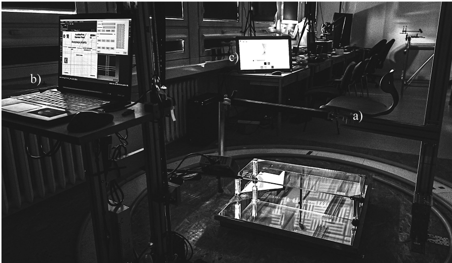
Fig. 1. The AutoMedPrint system prototype, a) 3D scanning rig; b) operator interface; c) user interface; station for 3D printing not shown
