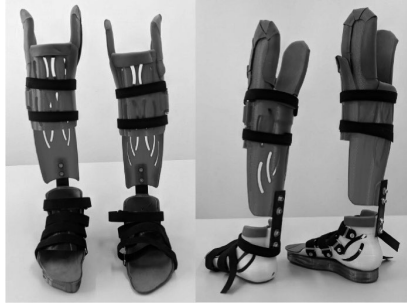
Fig. 7. The manufactured orthosis, design 2 – PET-G and nylon
