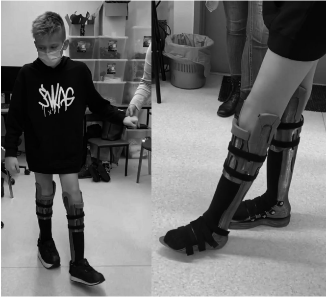
Fig. 12. Walking test of orthosis, version 3, with and without shoes
