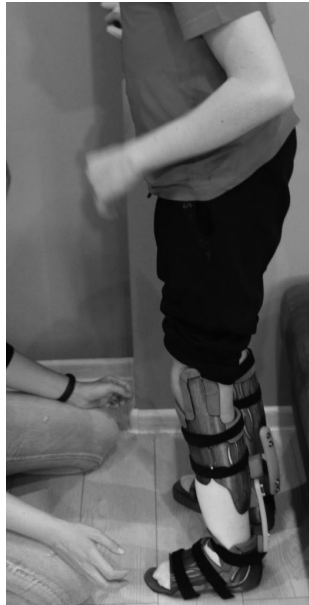
Fig. 10. Standing test of orthosis, version 1, visible bending of the nylon beam
