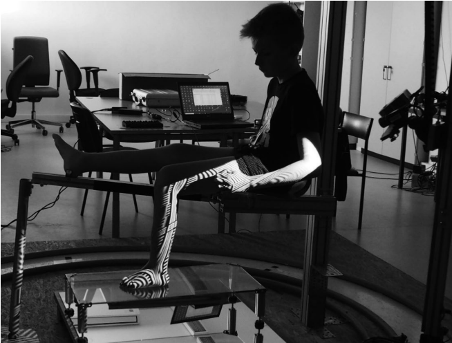
Fig. 2. 3D scanning of patient lower limbs using the AutoMedPrint system
