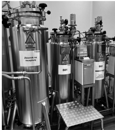
Fig. 10. Tanks used in the coating process (own study).
