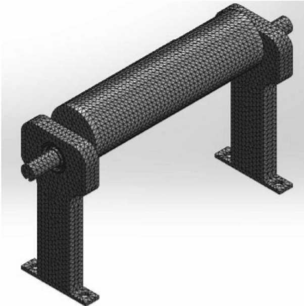
Fig. 5. The automatically generated grids (fine-grained meshes): A) the entire device, B) the single component.
