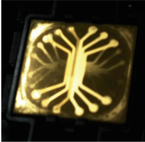
Fig. 8 Bio-Rad GLM SPR chip surface (with cartridge removed) shows vertical and horizontal strips corresponding to the 6 ligand and analyte channels. (Reproduced with permission from [101])
