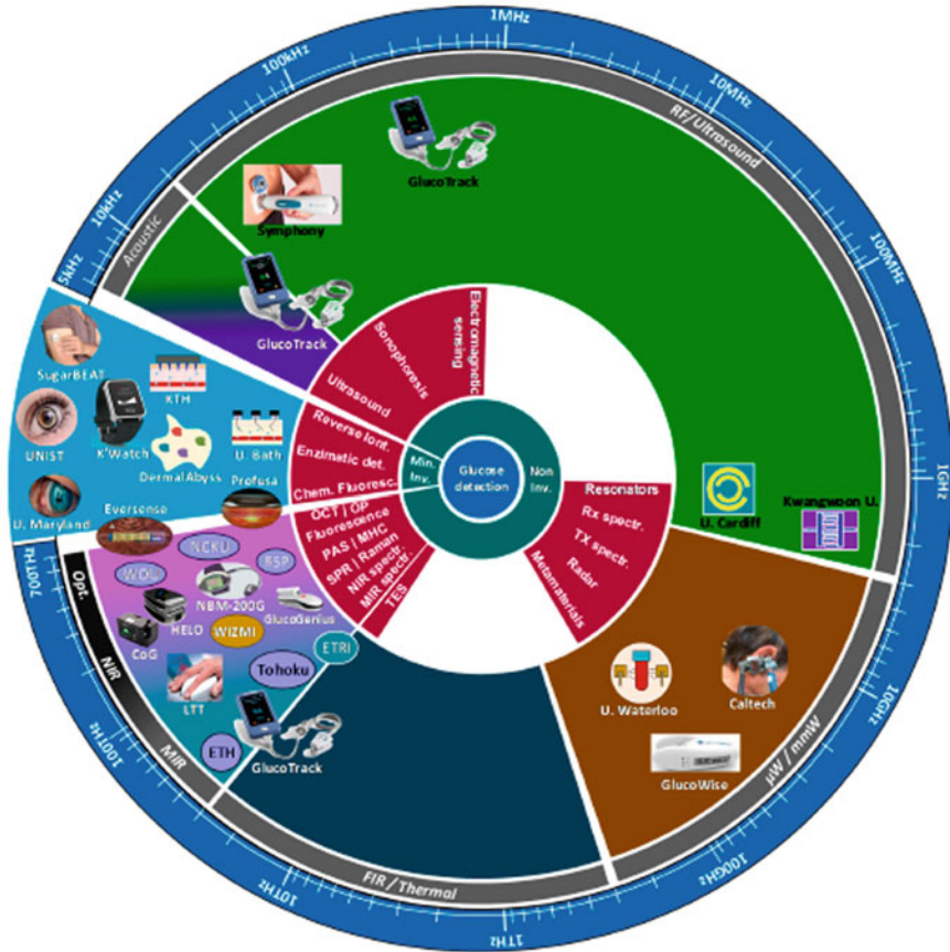
Fig. 11 The chart with location of non-invasive and minimally invasive methods and devices for glucose in the frequency spectrum. Reproduced with permission from [5] CC By © 2019 Gonzales et al., Licensee MDPI, Basel, Switzerland
