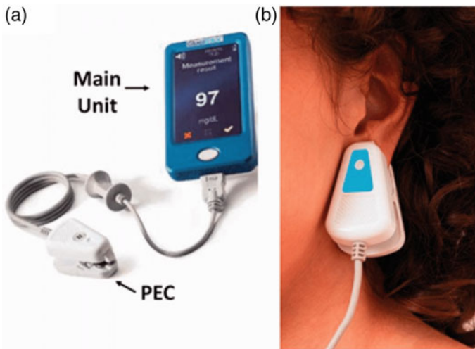
Fig. 3 GlucoTrack TM : non-invasive monitoring device [57]
