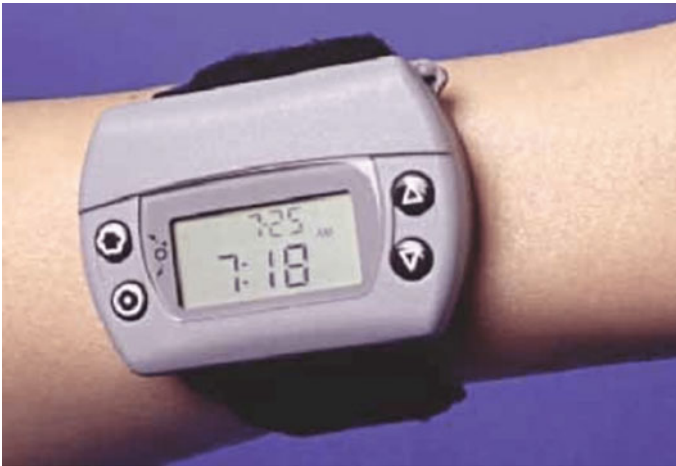
Fig. 2 The Biographer®: non-invasive glucose monitoring device [56]
