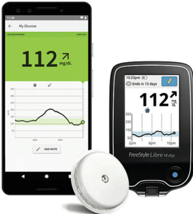
Fig. 4 Abbot FreeStyle® libre: glucose monitoring system [58]
