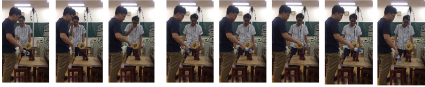
Fig. 6. Results of HUBOT-4.1 in robust and stable walking with sudden horizontal force
