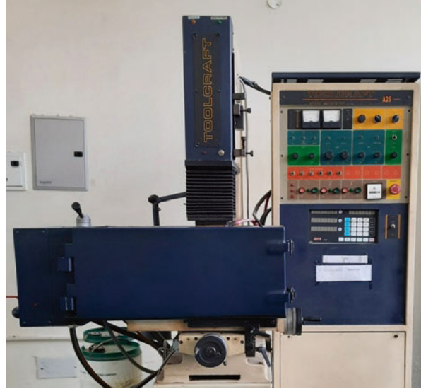
Fig. 1 Photograph of EDM (Courtesy: National Institute of Technical Teachers' Training and Research, Chandigarh)
