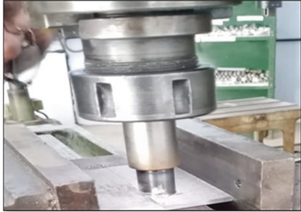
Fig. 1 Friction stir welding setup for joining 2 Mg AZ 31 alloy workpieces
