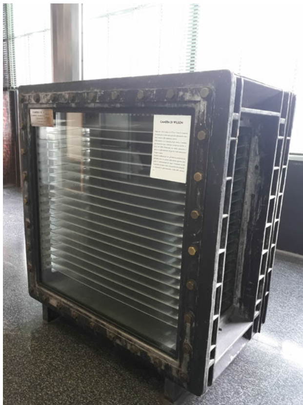
Fig. 7.1 The giant cloud chamber built by Ettore Fiorini, Riccardo Giacconi and Carlo Succi (Copyright: Leonardo Gariboldi)
