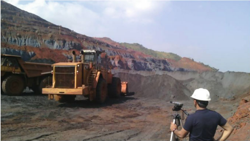
Fig. 1 Area noise monitoring in an opencast mine
