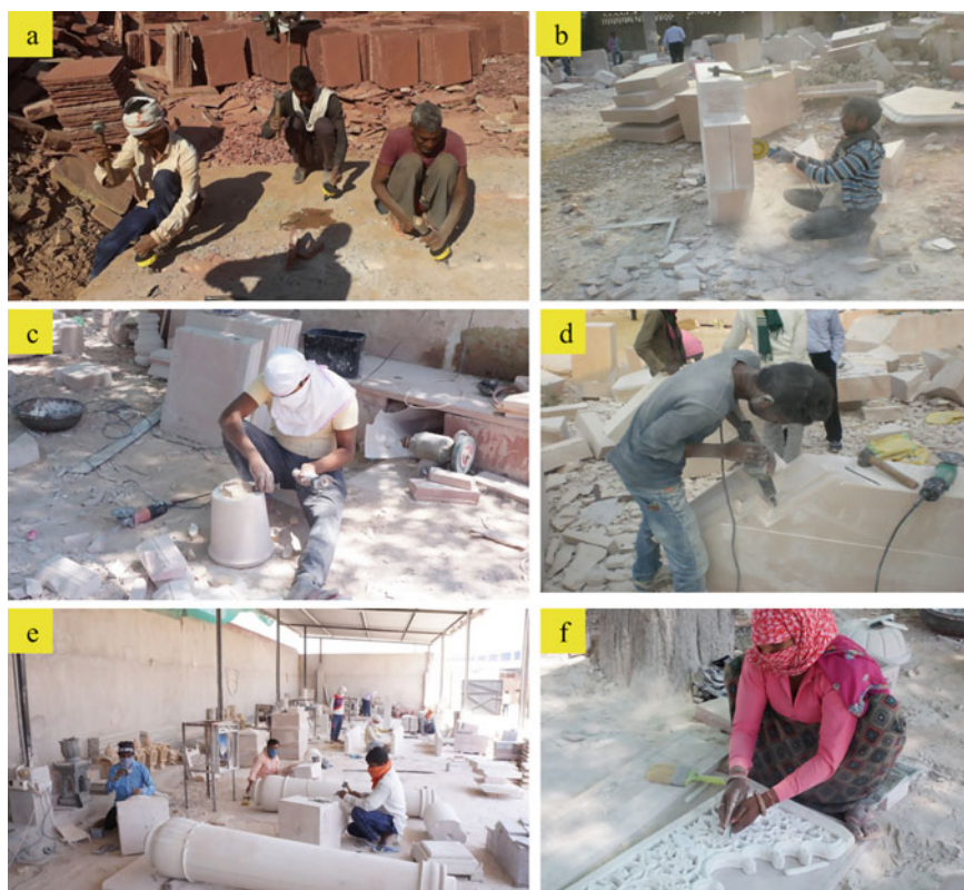
Fig. 1 a Chiseling a block of sandstone for extraction by manual mining, b Electric Hand Cutter being used in stone cutting, c Manual Chiseling, d Chiseling Operation with Electric Chisel, e Typical Stone carving Workshop in a large unit, f Manual rubbing and polishing
