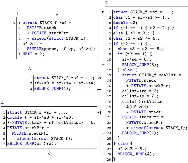
(c) Compiled RootPPL PCFG illustration. Some RootPPL constructs are omitted or slightly modified for readability. In particular, we omit the BBLOCK construct used in Fig. 4a. Instead, we illustrate the blocks as nodes in a graph, numbered by indices. The arrows indicate control flow between the blocks, with the incoming arrow to block 1 representing the call to f and the outgoing arrow from block 4 representing the return from f .
