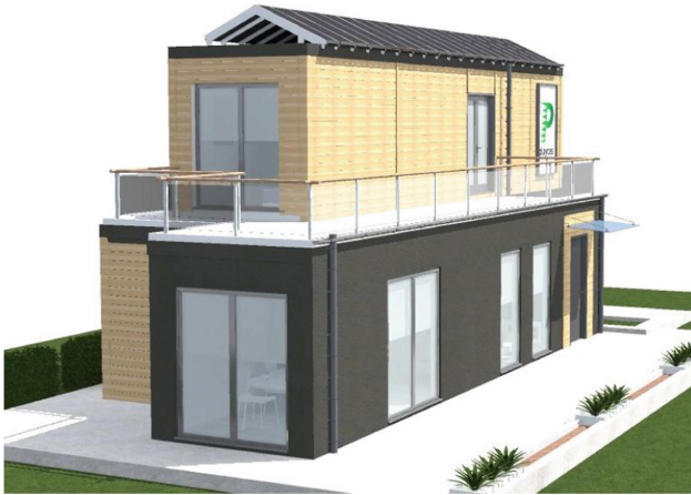
Fig. 4. Use of the sketchup program in the design of a 3D model of a house from prefabricated HQ 40-foot sea containers.
