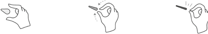
Fig. 1. Pointer pose gesture that can be used to point and select element [28].
