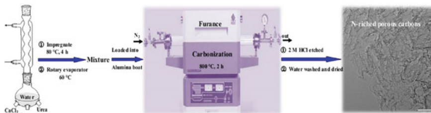
Fig. 4 Schematic illustration of the synthesis of N-rich porous carbons. Adapted with permission from Reference [39]. Copyright 2016 American Chemistry Society
