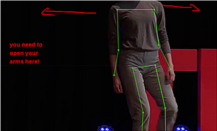
Fig. 2. MotionNotes with pose estimation. (Green: pose predictions; Red: manual annotation) (Color figure online).
