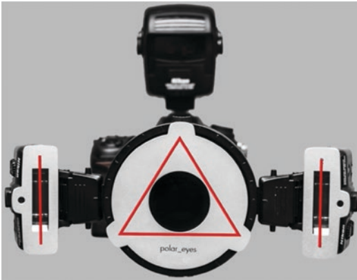
Fig. 5.21 Polar-eyes® cross-polarization filters. (Adapted from https://www.youtube.com/watch?v=uZwNKHnQyPw )
