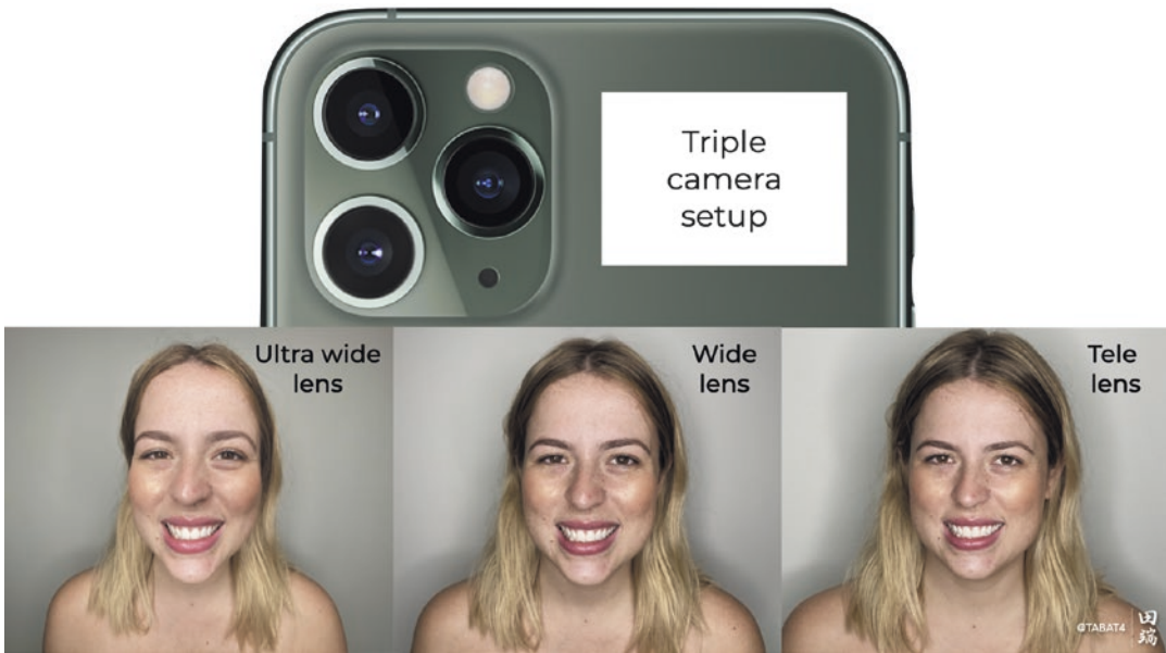
Fig. 5.6 Display of barrel distortion present in smartphones
