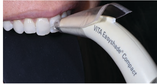
Fig. 3.33 Objective color measurement using Vita Easyshade V. (Photography courtesy of Bryce Brandfon, Franciele Floriani, and Nathalie Sawczuk)
