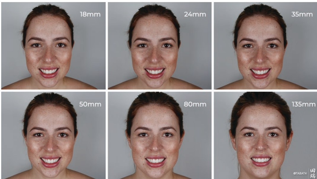
Fig. 5.5 Display of barrel distortion. Barrel distortion is usually present in most lenses, especially at wide angles. The distortion amount can vary, depending on the distance between camera and object, especially over short distances
