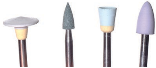
Fig. 8.8 Cups, discs, and flames silicon impregnated rubber. (Photography courtesy of Dr. Fernando Haddock)
