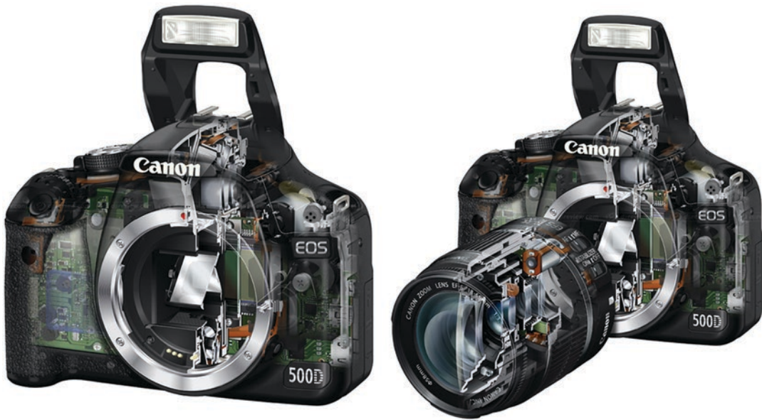
Fig. 5.3 Schematic illustration of a DSLR equipment. ( https://www.dpreview.com/articles/6579860130/canoneos500d )
