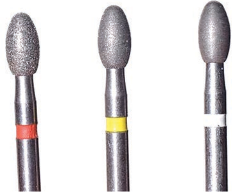
Fig. 8.6 Diamonds burs showing the difference in the grits from coarse to superfine. (Photography courtesy of Dr. Fernando Haddock)
