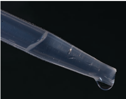
Fig. 9.4 BisGMA:TEGDMA (50:50 et%) monomer blend freshly removed from the bottle (Photography courtesy of Dr. Dayane Oliveira)
