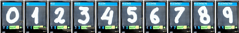
Fig. 4. ATmega2560 MCU integrating model, inference functions, graphics and touch screen functions in 24 KiB of program memory and 6 KiB of RAM.
