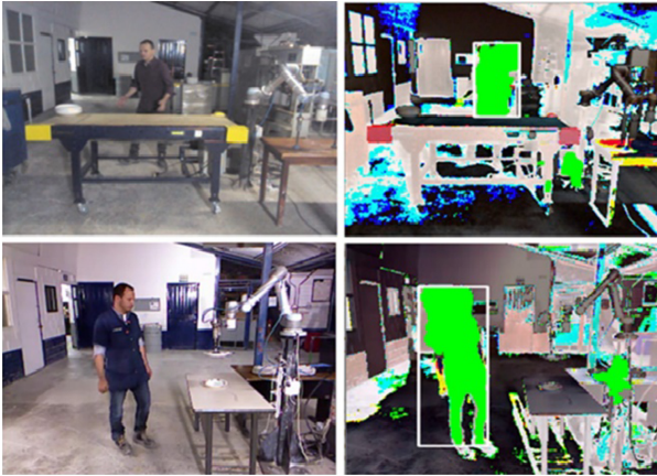
Fig. 2. Detection of relevant elements in RGB images in which 1 person appears. The OpenCV library for Python was used to apply filters, obtain contours, highlight in green and generate the ROI rectangles. The algorithm has been applied to images in the RGBD- DHaRIO dataset that contain only one person.
