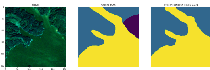
Fig. 5. Ground truth comparison against the predicted mask. Purple: open areas, Teal: forests, Yellow: water surface (Color figure online)
