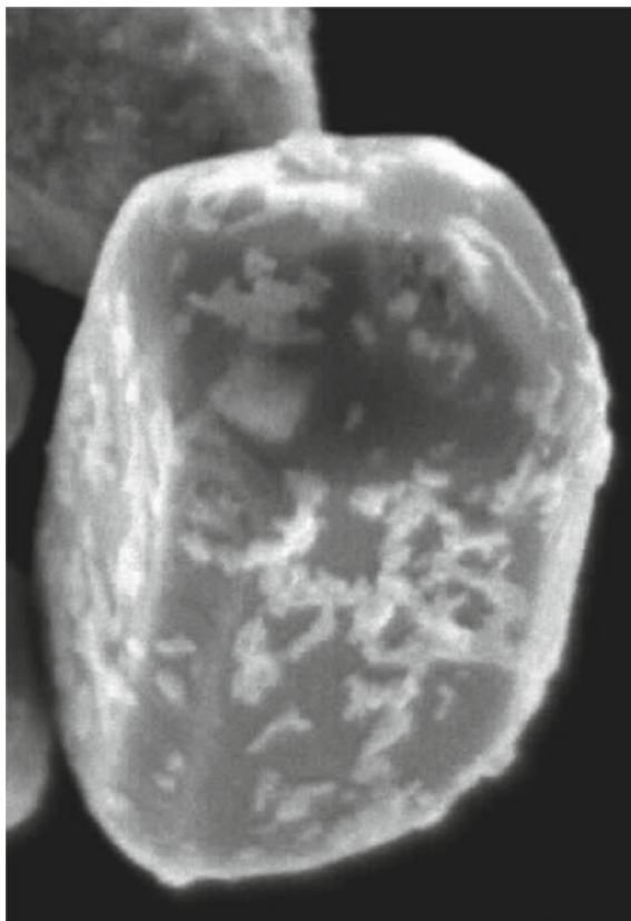
Fig. 7.4 SEM image of pigmentary \text{TiO}_2 coated with pseudo-boehmite particles
