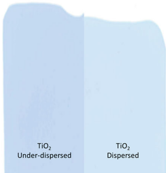
Fig. 13.22 Tinting strength test for \text{TiO}_2 . Difference in drawdown brightness is due to the degree of \text{TiO}_2 dispersion
