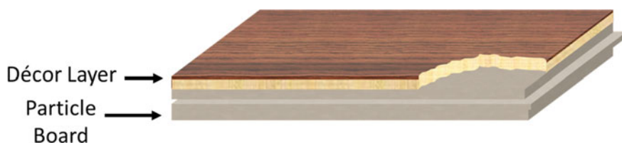
Fig. 18.1 Components of a laminate floorboard
