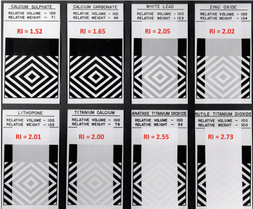
Fig. 18.2 Opacity contribution of different white powders to paint opacity
