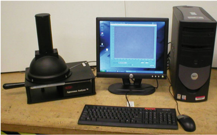
Fig. 18.13 Appearance analyzer employing a CCD camera to image 7\text{ cm} \times 8\text{ cm} laminate sample
