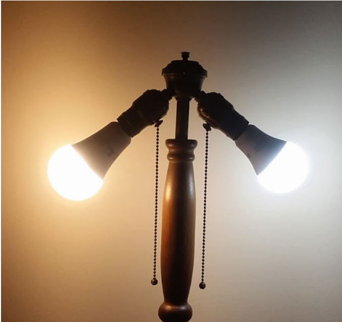
Fig. 5.10 Two “white” lights of various tones. Left—“soft warm” (color temperature 2700 K); right—“daylight” (color temperature 5000 K)
