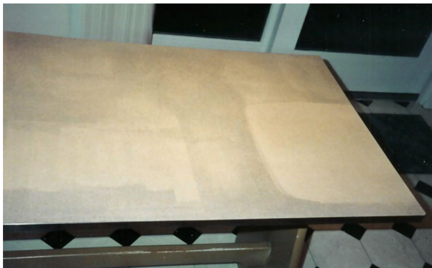
Fig. 14.18 Table with a paper laminate surface after 1 day exposure to sunlight. Here the tabletop was partially covered, resulting in light regions (original color) surrounded by dark regions (photo-grayed)
