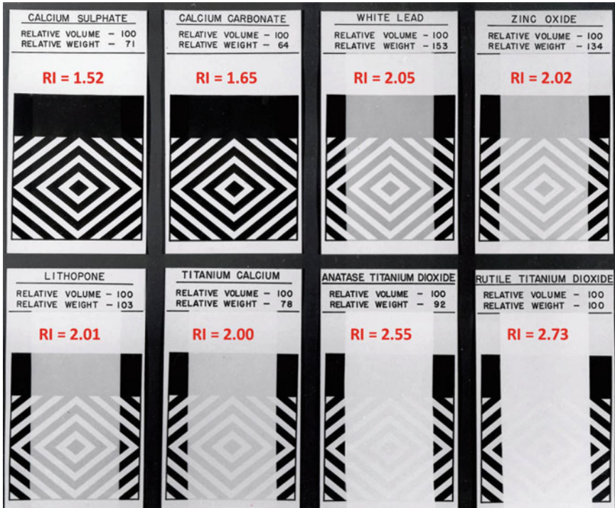
Fig. 3.7 Opacities of paints made with different white particles. All paints are at the same thickness and have the same volume concentration of particles [5]
