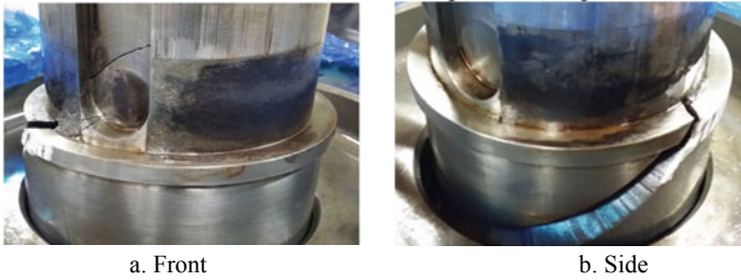
Fig. 3 Fatigue fracture of reducer shaft [18]
