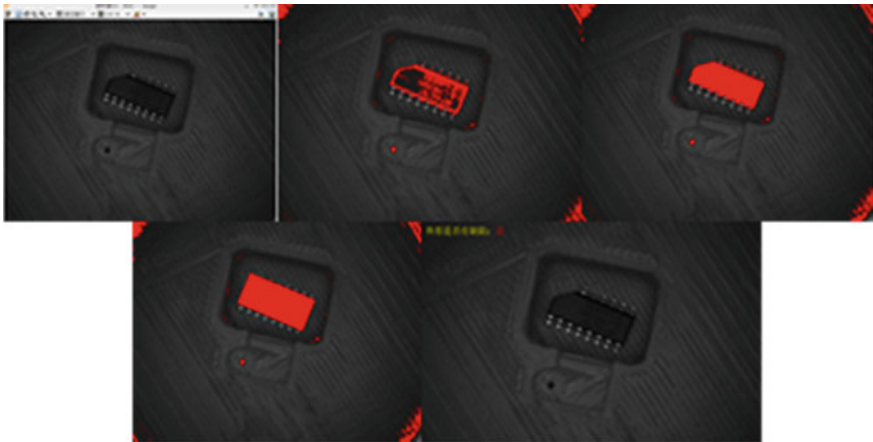
Fig. 8 Profile defect detection process
