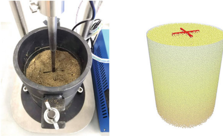
Fig. 14 Vane shear test and simulation model
