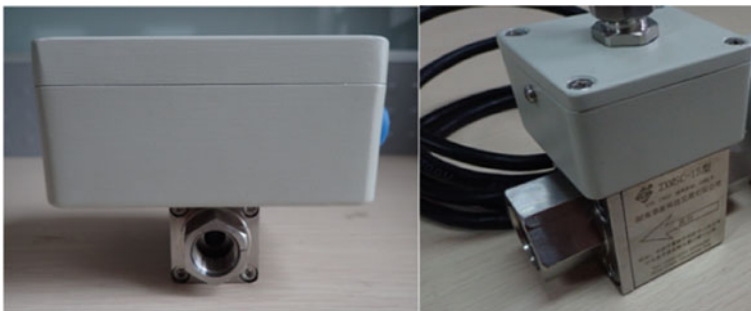
Fig. 1 The inductive metal debris sensor prototypes we developed (Left: for 8 mm diameter pipe, Right: for 15 mm diameter pipe)
