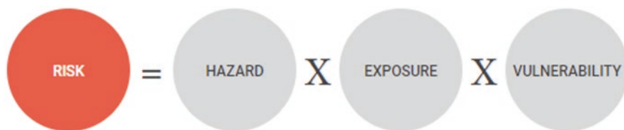
Fig. 12.3 The classical risk definition still places hazard first. Even though the definition stresses on interactions, the conceptual model (a graphical representation of the definition) is still linear. (Source: https://www.preventionweb.net/disaster-risk/risk/disaster-risk/ (2020))
