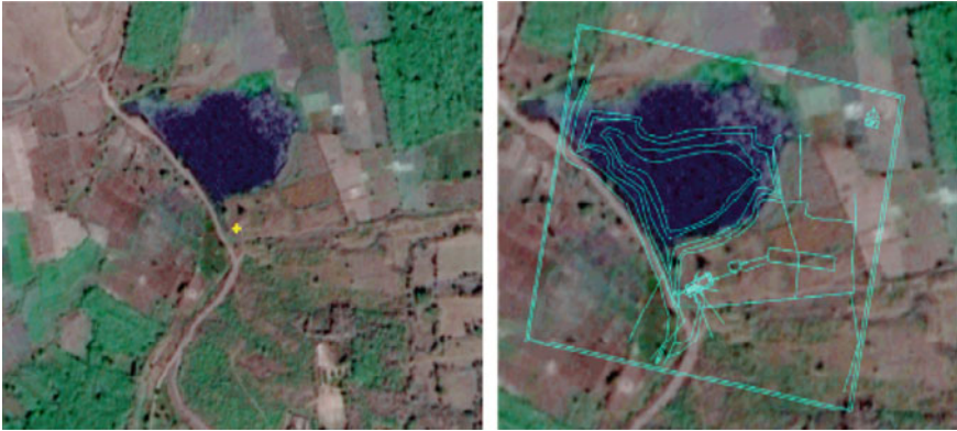
Fig. 23.8 Protected boundary delineation using total station data: Praneshvara temple, Shimoga
