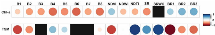
Fig. 9.2 Correlograms explaining the correlation (r) of Chl- a (upper plot) and TSM (lower plot) with S2 MSI bands (8 bands), spectral indices derived from C2RCC processing and band ratios derived (see Table 9.1). Blacked out boxes indicate insignificant correlation at 95% significant level
