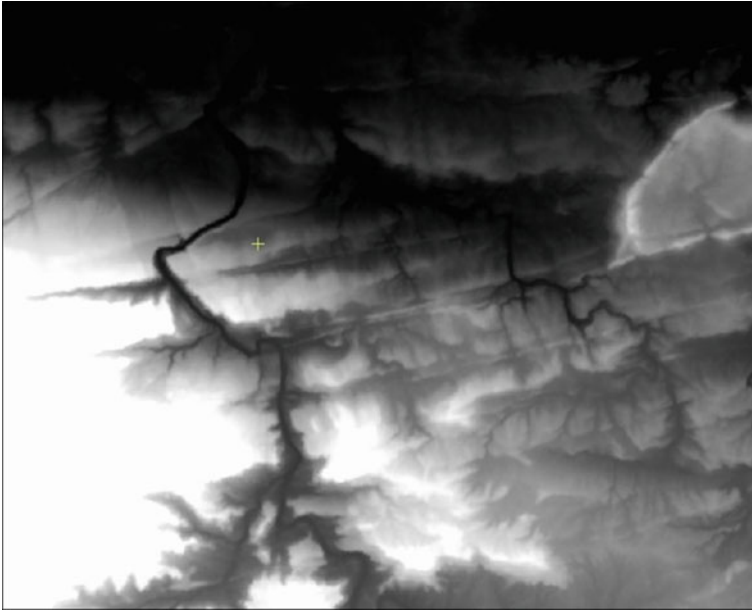
Fig. 18.16 Output of the process of DEM accuracy improvement using I-sigma-based filtering of outliers by using multi-temporal stereo data. Example of Mahabaleshwar area, Maharashtra
