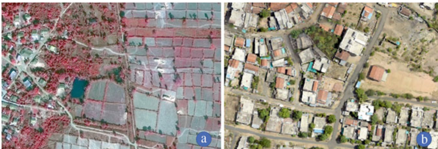
Fig. 21.1 a Satellite data (50 cm), b UAV data (5 cm)—high-resolution data form the base of all land property records and their uses
