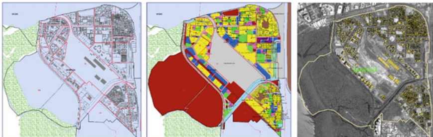
Fig. 21.6 A sample digitized city survey cadastral map with land use attributes and satellite data overlay
