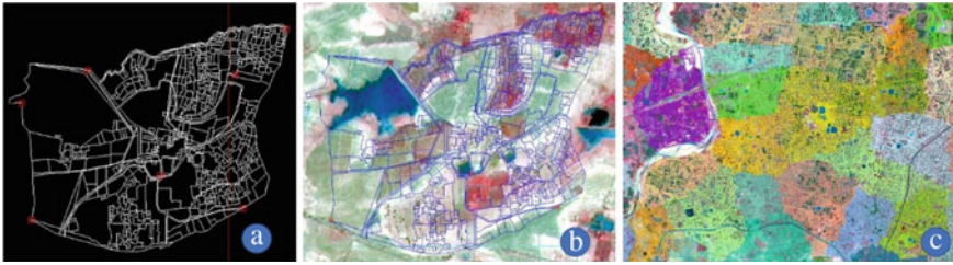
Fig. 21.7 Georeferencing of cadastral map— a Vectorized and attributed village map with tie-points, b georeferenced village on the satellite data, and c mosaiced multiple villages cadastral maps on satellite data
