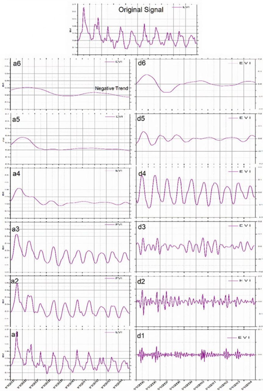
Fig. 29.4 Wavelet decomposition representing negative trend in long-term EVI data (2005–2014) where a and d indicated approximation and detailed components respectively
