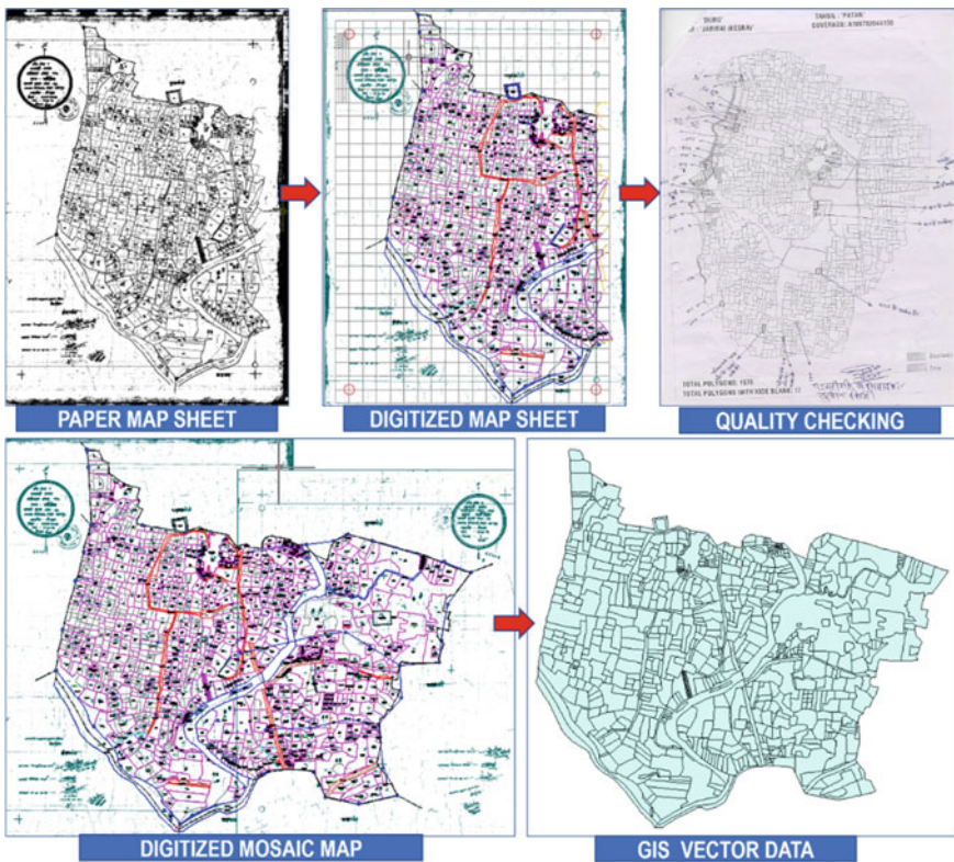
Fig. 21.5 Cadastral map grid referencing, vectorization, mosaicking, and GIS format conversion
