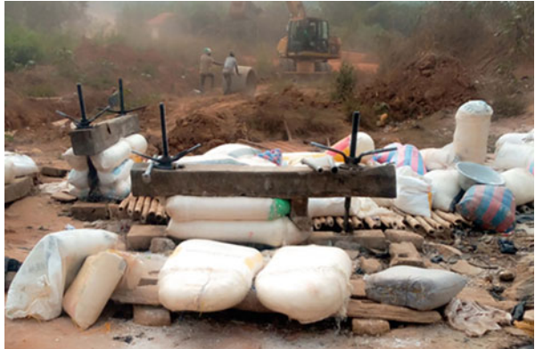
Fig. 5 Crushed cassava dough bagged in sacks and placed under pressers to extract starch and water (Photo © Jacqueline Zakpaa)
