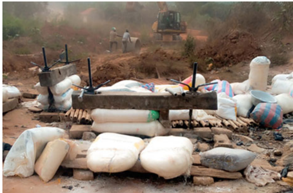
Fig. 5 Crushed cassava dough bagged in sacks and placed under pressers to extract starch and water (Photo © Jacqueline Zakpaa)
