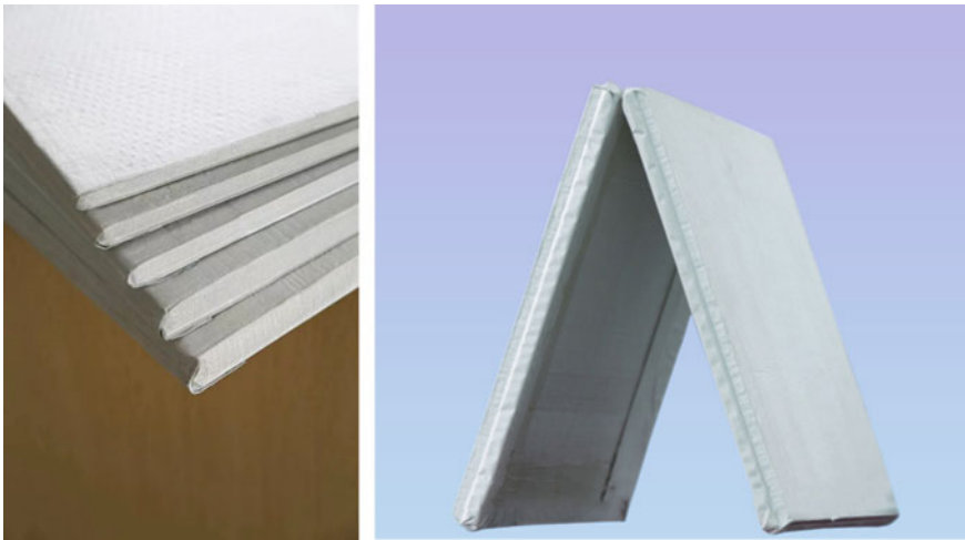
Fig. 11.12 Photograph of VIP with fiberglass cloth envelope
