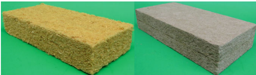
Fig. 6.1 Flexible wood fiber batt for cavity insulation (left) and wood fiber board for exterior wall insulation systems (EIFS)
