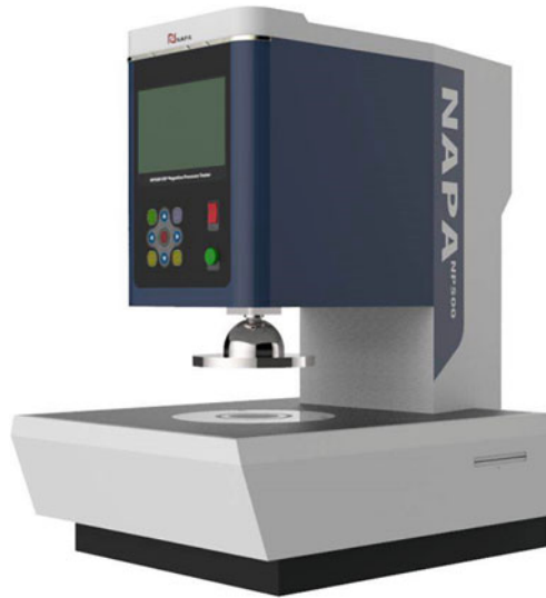
Fig. 11.26 Test equipment for measurements of the VIP’s inner pressure (NAPA, made by NUAU)
