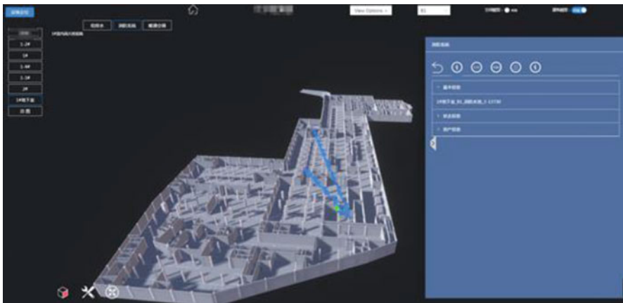
Fig. 4.13 Water tank and route for fire hydrant in basement. Source: SpaceBox technical whitepaper
