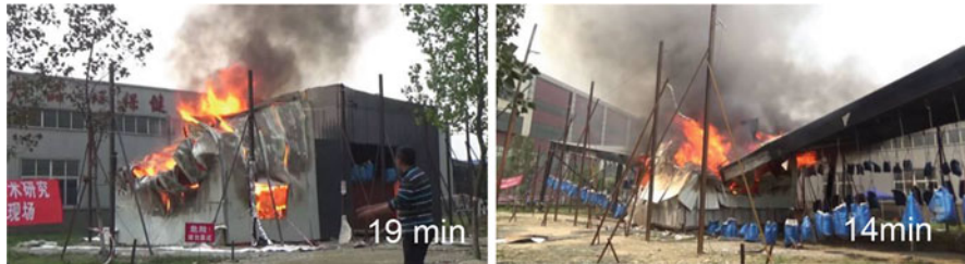
Fig. 13.23 Structural collapse in Test 1 and Test 2
