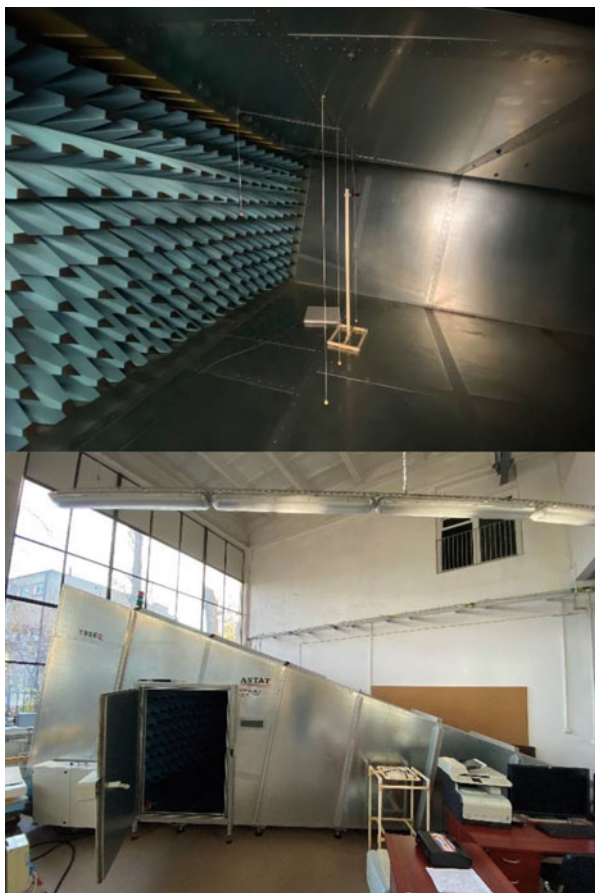
Fig. 11.18 Interior of GTEM chamber of the ITB Fire Testing Laboratory, Warsaw, Poland
