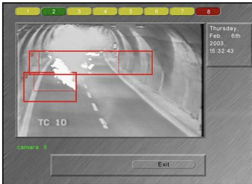
Fig. 4.2 Fire detection system based on the image processing technology (source: website)
