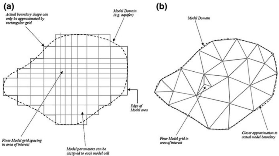
**Fig. 3.5** Illustration of (a) finite difference method (FDM) and (b) finite element method (FEM) (NGCLC 2001)
