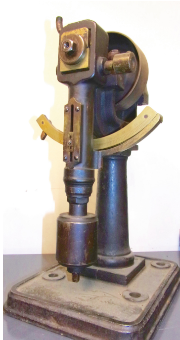
Fig. 6. Thurston’s Lubrication Testing Machine. This machine was described in Thurston’s 1883 Three Volume book Materials of Engineering [14].
