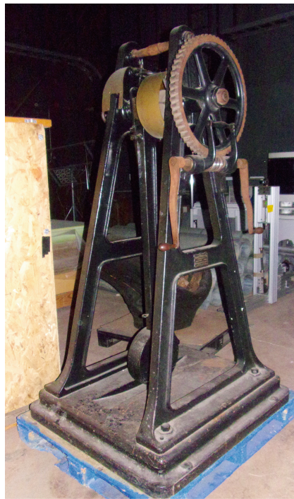
Fig. 3. Photograph of autographic torsional testing machine in the Thurston Collection at Cornell University, Ithaca, NY. USA.
