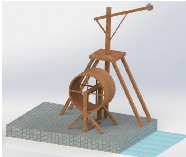
Fig. 9. Virtual mock-up of the port crane.
