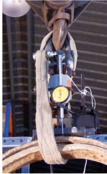
(b) Close-up of the eyebolt fastening, touch probe and safety system
