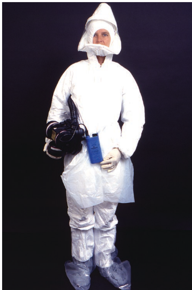
Fig. 29.2 Powered air-purifying respirator. This 1995 image depicts an anterior view of a laboratory technician wearing garments, usually worn by field techs, including a disposable white coverall, a disposable plastic apron, head covering, latex gloves, and foot coverings, and is equipped with what is known as a 3 M™ Breathe Easy™ Powered Air Purifying Respirator, PAPR. Though this 3 M™ PAPR can be equipped with either a biological rated filter cartridge, or a chemical rated filter cartridge, this outfit is rated only for a biologic interaction, and not chemical. (This image # 13161 accessed on 4/3/2021 at URL https://phil.cdc.gov/phil/home.asp )
