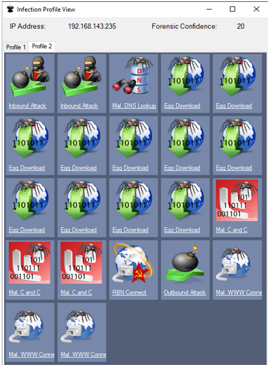
Fig. 4. Infection Profile View for one of the chosen IP addresses that are of interest to the user. Each infection profile view may have several infection profiles, each consisting of a list of icons that symbolize the various evidence classes (e.g., inbound attack, egg download, connection to malicious Command and Control (C&C) Server, connection to Russian Business Network (RBN), or outgoing attack)). Infection Profiles provides a quick overview for the operator what has been going on with the network asset in question and where the attack stands. This will enable the user to quickly decide where to put his attention and act on isolating network nodes to limit the damage and contain the exposure.
