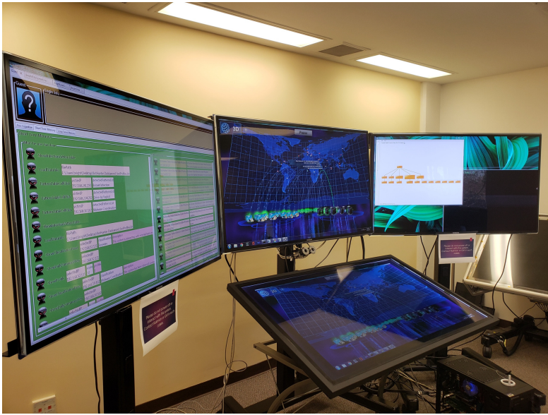
Fig. 1. A bRIGHT workstation consisting of a touch table with proximity detection for positioning controls under the hands of users. The center monitor has a gaze tracking system mounted on the bottom that records what the user is looking at. The user is working with a cybersecurity application that is rendered on the center monitor. The left monitor visualizes the recorded raw data regarding the user's interactions with the application (what the user did) and the user's gaze (what the user looked at). The right monitor visualizes the generated user context model that represents the user's interest at any given time.
