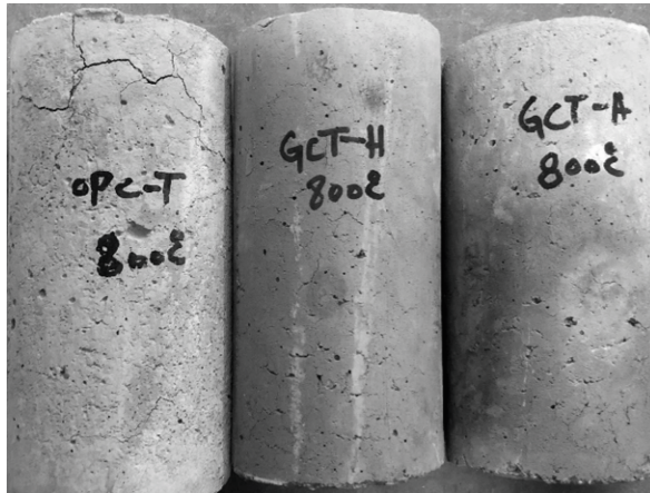
Fig. 1. Cracks of GPC and OPC concrete after exposure to 800 °C (Hassan et al. 2020b)
