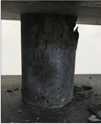
Fig. 4. Compression test on cylinder specimen
