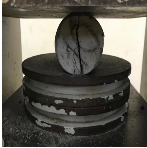
Fig. 5. Tensile test on cylinder specimen
