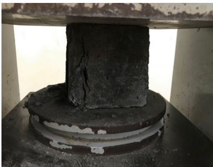
Fig. 2. Compression test on cube specimen
