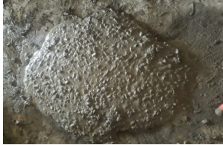
Fig. 1. Slump flow test
