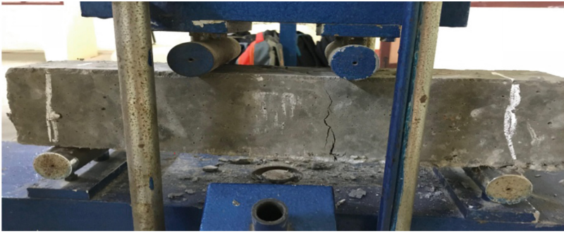
Fig. 12. Modulus of rupture test set up
