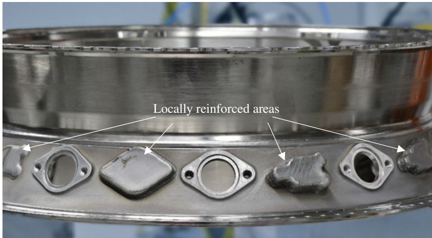
Fig. 13.6 Aerospace component with locally reinforced areas manufactured by Hybrid AM (Günter Neumann et al. 2021)
