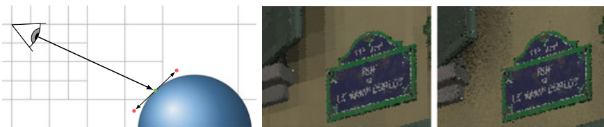
Fig. 6 Jittering trades quantization artifacts for noise. Left: Note that the resolution s(k) at the jittered location (red) may differ from the one of the original location (green). Spatial jittering hides otherwise visible quantization artifacts (middle): The resulting noise (right) is more amenable to the eye and much simpler to remove by a secondary filter
