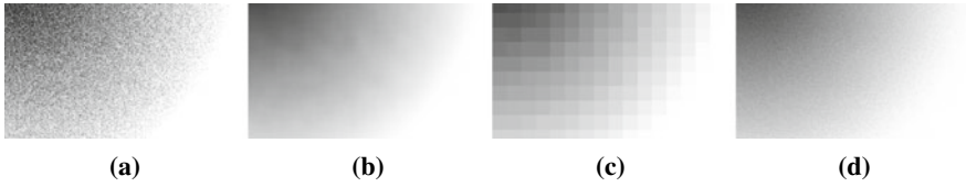
Fig. 7 Two-dimensional example for averages in voxels: The noisy input (a) is filtered in each vertex by path space filtering (b) yielding a splotchy result that is difficult to filter. Instead, the new method filters in each voxel, resulting in block artifacts (c). Additionally jittering before accumulation and lookup resolves the artifacts in noise that is simple to filter (d)
