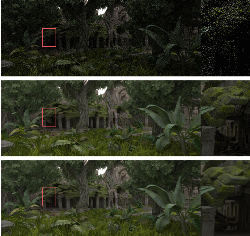
Fig. 1 Path tracing at one path per pixel (top) in combination with hashed path space filtering (middle) very closely approximates the reference solution using 1024 paths per pixel (bottom) and does so with an overhead of about 1.5 ms in HD resolution. Scene courtesy of Epic Games
