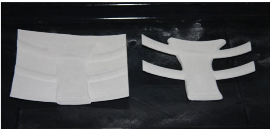
Fig. 8.5 Finished original mold obtained by 3D printing process
