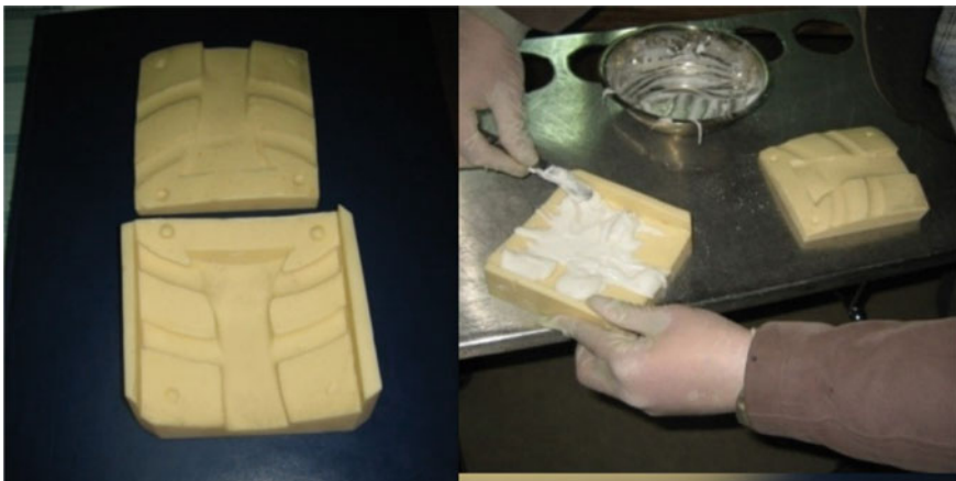
Fig. 8.6 Mold obtained on the basis of the original (left) and filling of the mold with prosthetic material (right)
