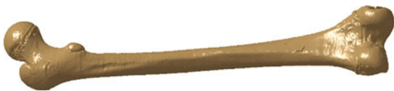
Fig. 17.4 Polygonal model of the femur, after the removal of the unnecessary portions (Korunovic et al. 2010)
