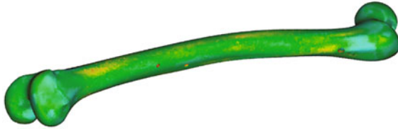
Fig. 17.15 FE model of femur with material properties assigned (shown in different colors). Screw holes are also visible on the model. Lowest values are shown in light blue, while the highest ones are shown in red (Korunovic et al. 2015)
