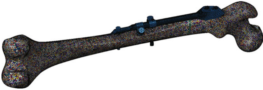
Fig. 17.16 Final FE model of femur-SIF assembly, containing the fracture zone (Korunovic et al. 2015)
