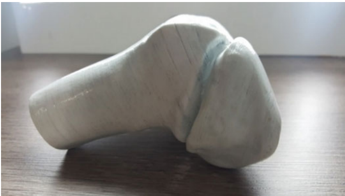
Fig. 14.9 The 3D printed bone model with FDM technology in white ABS, distal femur and fragment of the lateral femoral condyle
