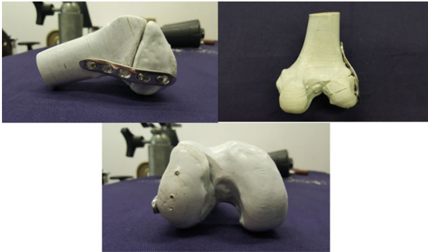
Fig. 14.10 3D printed bone model fixated with the plate and screws on the anatomical model (lateral side of distal femur)
