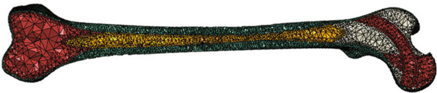
Fig. 17.12 The zones and the corresponding FE mesh of the femur model. Green: trabecular bone, E = 12.7 GPa. Red: cancellous bone (denser trabeculae), E = 0.3 GPa. White: cancellous bone (sparser trabeculae), E = 0.07 GPa. Yellow: Bone marrow, 1 MPa (Korunovic et al. 2010)
