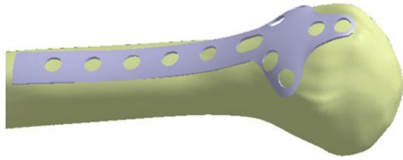
Fig. 6.29 Assembly of the customized plate solid model and surface model of the humerus. (Reproduced from Rashid 2018)
