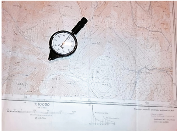
Fig. 2. The special tool “opisometer” was used to measure the lengths of microrelief shapes on maps in scale 1: 10 000.
