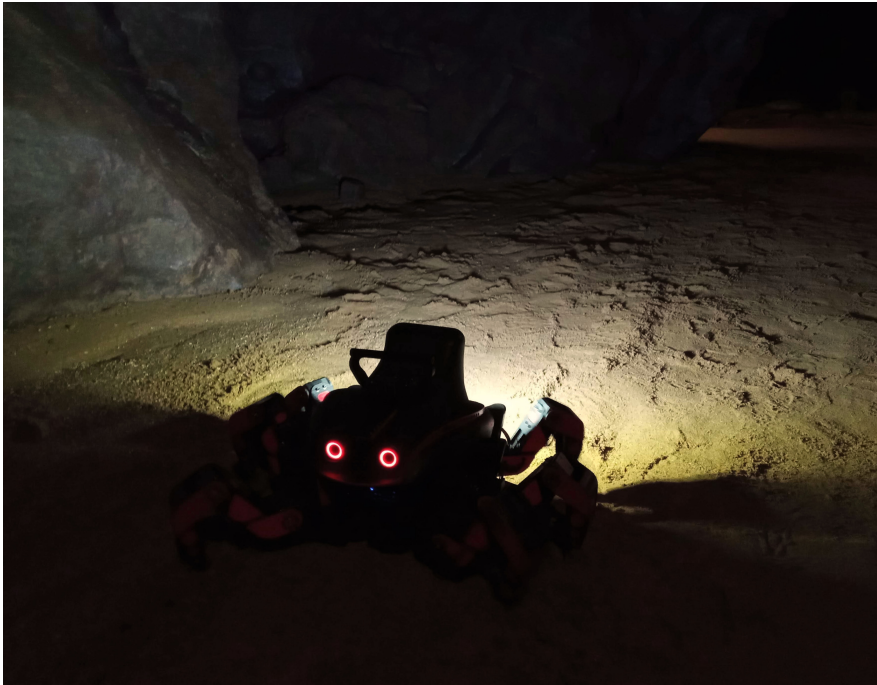
Fig. 1. The used hexapod walking robot in the experimental deployment of the proposed method in the Bull Rock Cave, where it builds elevation map and collects the dataset.
