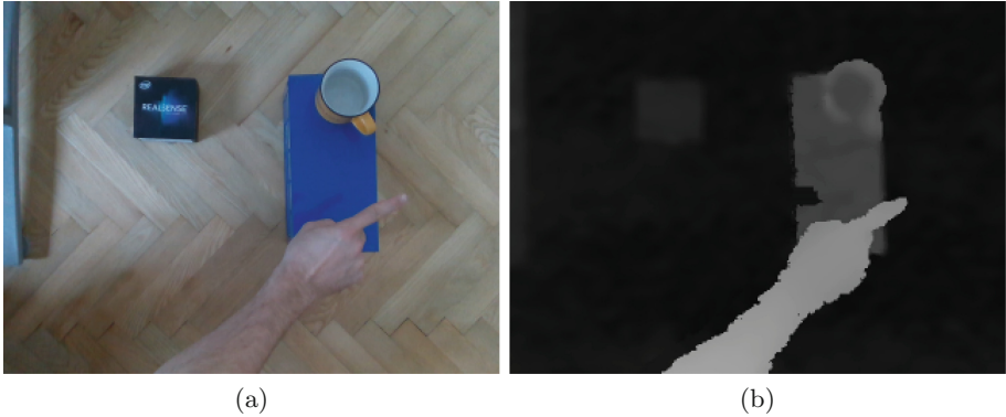
Fig. 5. Image captured with a real RGB-D camera mounted 1 m above the ground, scene includes objects of basic shapes and the hand: (a) RGB image of the scene, (b) depth image with applied hole filling filter.
