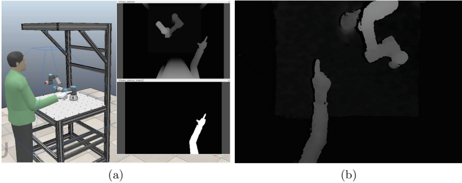
Fig. 7. Experimental workplace with the robot Universal Robots UR3: (a) Simulation environment CoppeliaSim with imported workplace including robot UR3. Figurine has a hand with pointing gesture mounted to the right arm. Output of the generator are depth (upper) and label (bottom) images, (b) image captured with real camera at the workplace in the laboratory.
